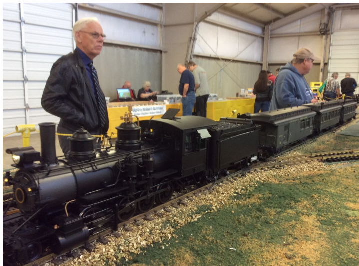
A show visitor and Jerry Madsen stand next to the maiden outing of Don MacLaren's Bachman C19 which he bought at the convention in Denver. Don installed an Airwire drop-in receiver, battery, and Phoenix sound system. It ran about 2 hours on a charge.
